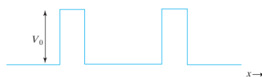
FIGURE 2.6 Potential energy for a particle in a one-dimensional box of finite height and thickness.
